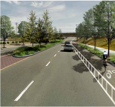
Medians, trees, bicycle lanes, and sidewalks improve the appearance and function of a standard arterial.
